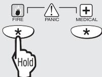
The Keypad Fire alarm function is disabled by default, and must be enabled by your installer.
